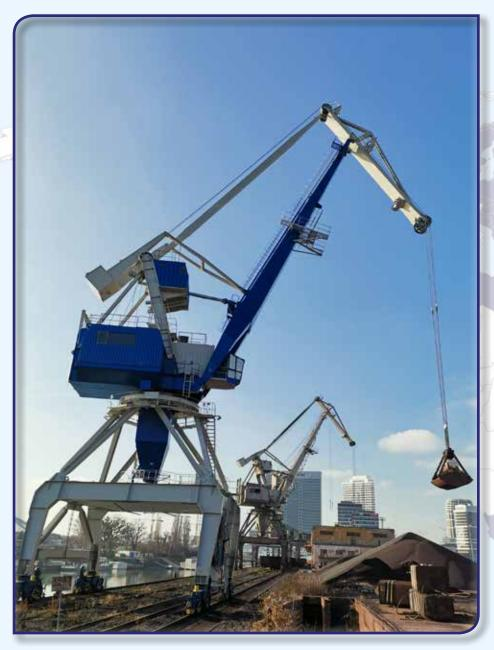
16/27 t x 33/21 m – capacity GANZ-type double-jib level-luffing portal crane
