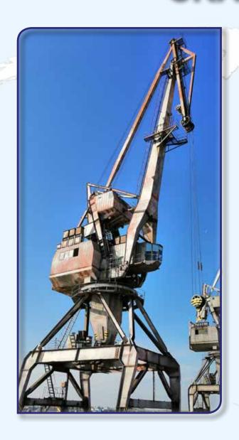
16/27 t x 33/21 m – capacity GANZ-type double-jib level-luffing portal crane
