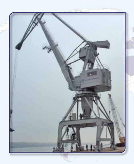
16/27 t x 33/21 m – capacity GANZ-type double-jib level-luffing portal crane
