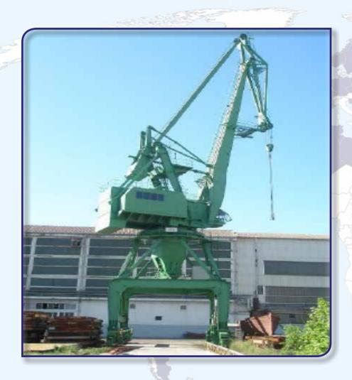
16/27 t x 33/21 m – capacity GANZ type Double-Jib Level-Luffing Portal Crane
