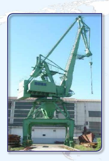
16/27 t x 33/21 m – capacity GANZ type Double-Jib Level-Luffing Portal Crane
